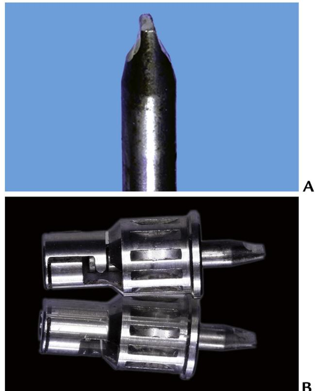
**Figure 1.** A, Round bur after modification. B, Assembly of custom screwdriver.
